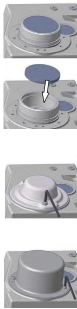
Figure 3-12: Fitting the covers, Option SH, Option H, and Option H66
