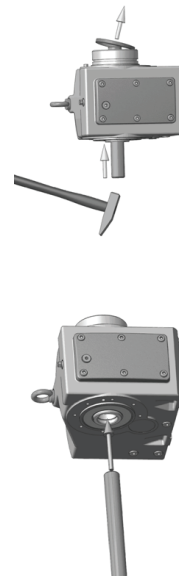
Figure 3-5: Removing the factory-fitted closing cap
