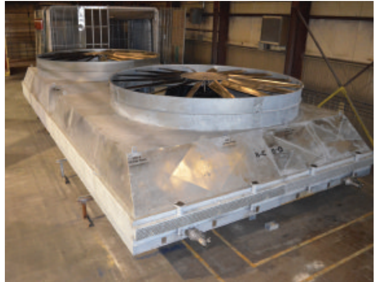
■ A two-fan Model E horizontal cooler is in process in the large cooler assembly line at Alfa Laval ACE's plant in Broken Arrow, Oklahoma.
