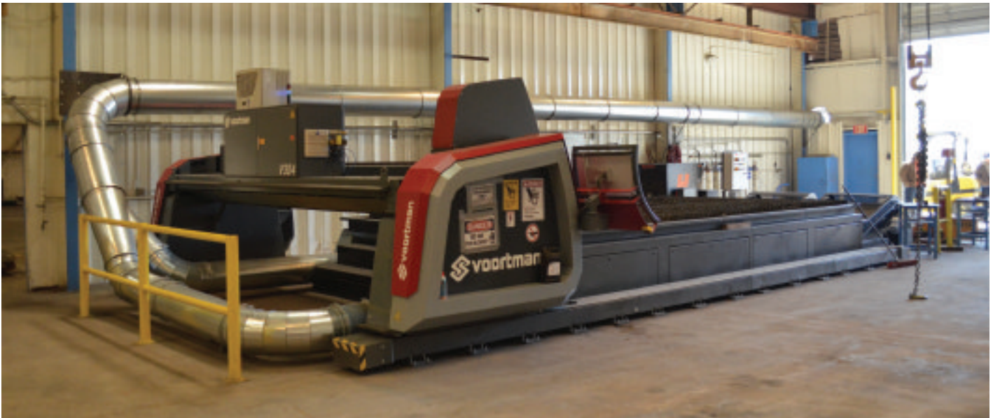
■ This new CNC burn and bevel table, installed in Alfa Laval ACE's Broken Arrow, Oklahoma, facility last year, increased productivity and throughput by a factor of three.
